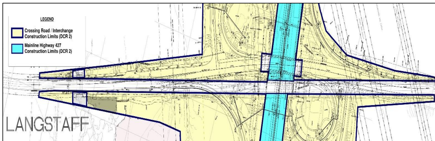
Figure 12: Langstaff Road Construction Limits & Final Alignment
